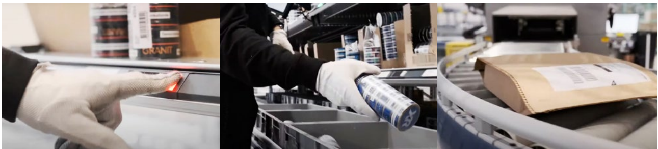
Figure 20: Haypp Group's automated warehouse in Stockholm with pick-by-light function
